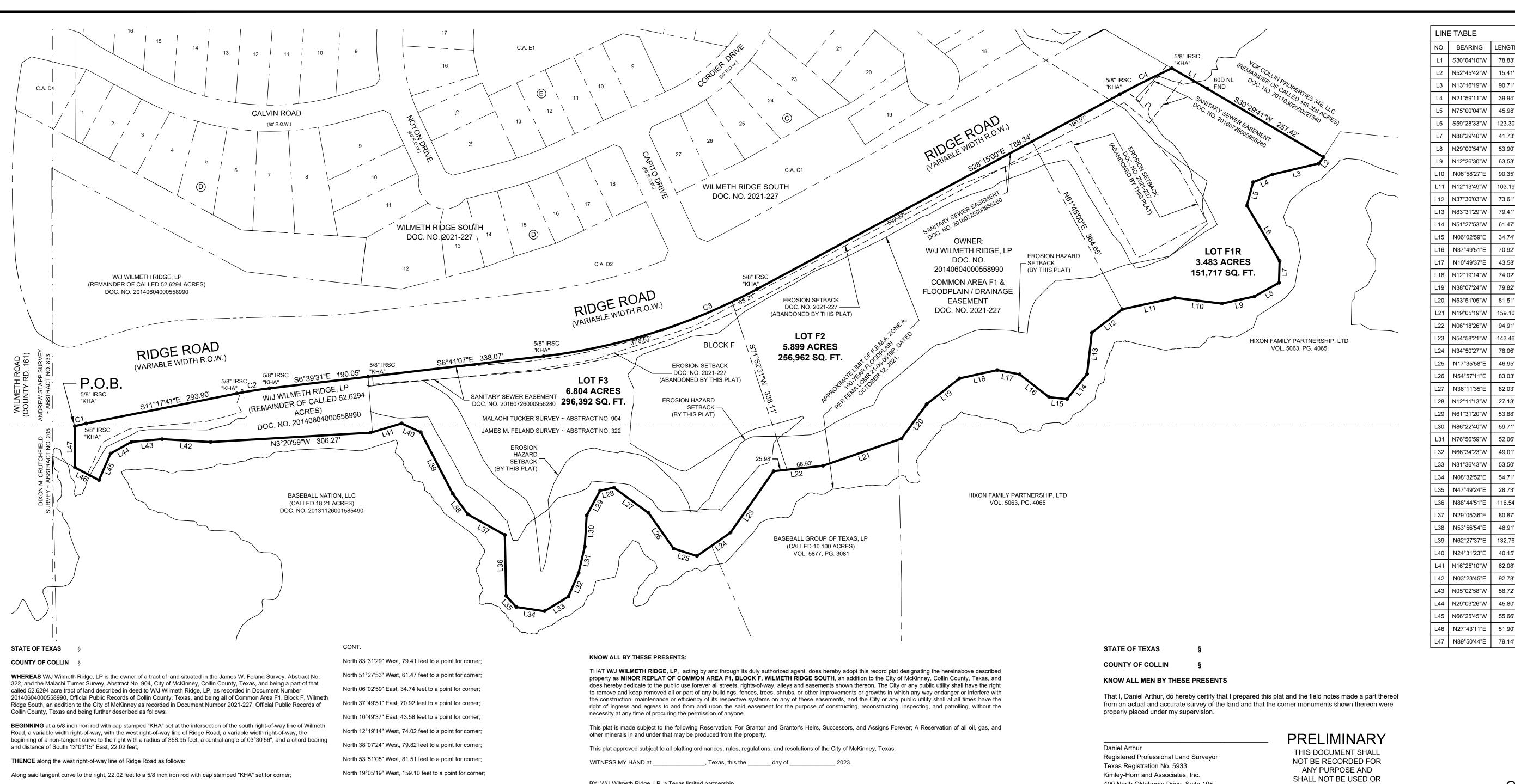
South 11°17'47" East, 293.90 feet to a 5/8 inch iron rod with cap stamped "KHA" set for corner, the beginning of a tangent curve to the right with a radius of 783.88 feet, a central angle of 04°36'36", and a chord bearing and distance of South 08°59'29" East, 63.05 feet;
