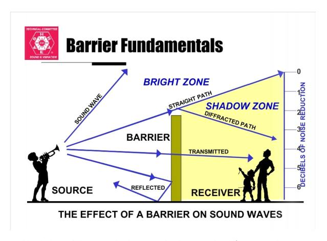
A sound barrier is a solid structure that intercepts the direct sound path from a sound source to a receiver. It reduces the sound pressure within its shadow zone. Barriers should be constructed of solid, not porous material. Material includes pre cast concrete. We are providing a concrete block sound barrier and a new brewery building that will act as a sound barrier.
