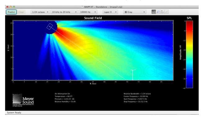
Speakers are directional and the direction of sound can be fine-tuned as required to provide a cone of sound to provide a good listening experience for events, but lower levels of sound for surrounding residences.
